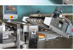
The system's incline design lets gravity assist in keeping stacked product in place
