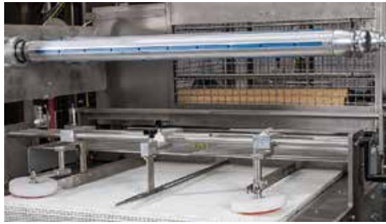
Pneumatic film spindles expand to hold the film in place without damaging the cardboard core and allow for plastic cores.
