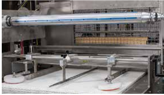
Pneumatic film spindles expand to hold the film in place without damaging the cardboard core and allow for use of plastic cores.
