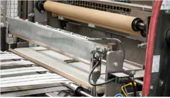
Seal bar design offers precise heat control and fast impulse sealing technology. Narrower transfer allows for running smaller product across the bar.
